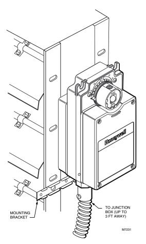
Fig. 6. ML6275 Actuator standard electrical connection.
